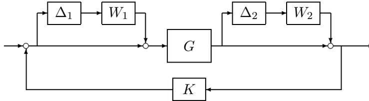
FIGURE 2. Feedback stabilization with uncertainties in observation and control channels.
